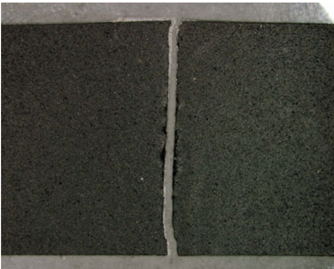
FIG. 6—Test set 8C, 3M Tartan™ 1710, 7 mil vinyl electrical tape nicked and then hand-torn by preparer B.
